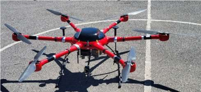
Figure 1. Haemus Hexacopter Skylle 1550 used in the experiments.
