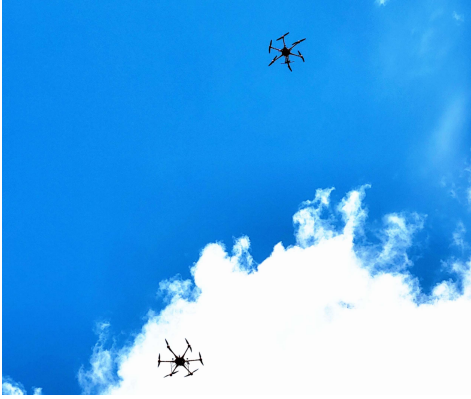
Figure 2. The transmitting drone (top) and the measuring drone (bottom) in flight (as seen from the ground).
